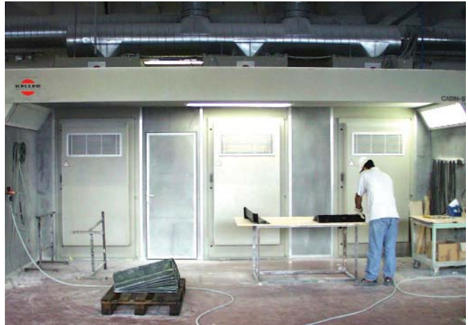
Manual grinding processing of glass fibre reinforced plastic components
